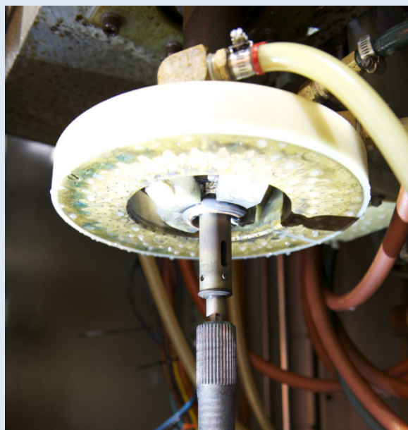
A six-axis robot places axle shafts in the induction heat treating scanner. The process induces a very high current in the shafts, which instantly heats them. Rapid cooling or quenching hardens them.
