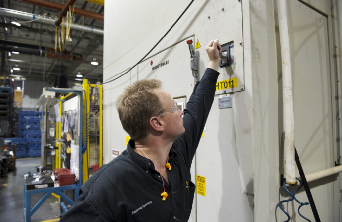
The back of the fixture houses the power to drive the heat treating process. Leigh Copp de-energizes the entire system before going inside to take measurements.
