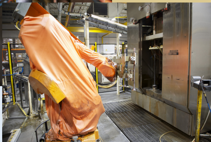
A six-axis robot places axle shafts in the induction heat treating scanner. The process induces a very high current in the shafts, which instantly heats them. Rapid cooling or quenching hardens them.
