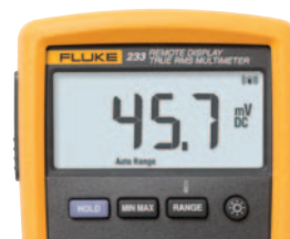
Detachable wireless display on Fluke 233 Remote Display Digital Multimeter.
